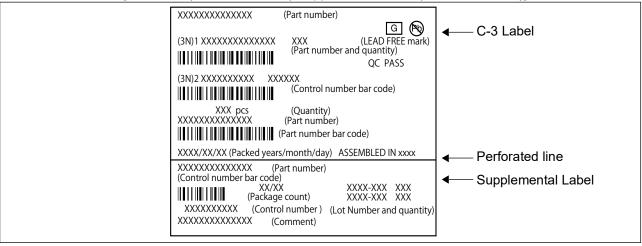
Label II:Moisture Barrier Bag (It sticks it on the Aluminum laminated bag) only for MB85RC16VPNF-AWERE2
