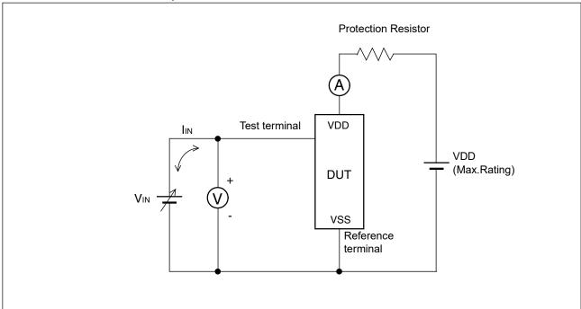
Note: The voltage  $V_{IN}$  is increased gradually and the current  $I_{IN}$  of 300 mA at maximum shall flow. Confirm the latch up does not occur under  $I_{IN}=\pm300$  mA. In case the specific requirement is specified for I/O and  $I_{IN}$  cannot be 300 mA, the voltage shall be increased to the level that meets the specific requirement.
